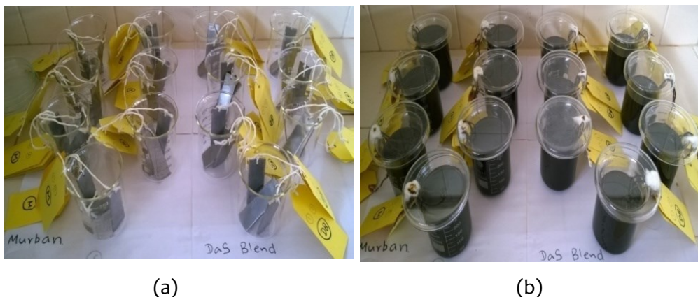
Figure 3: (a) Immersion of metal coupons and (b) apparatus.
